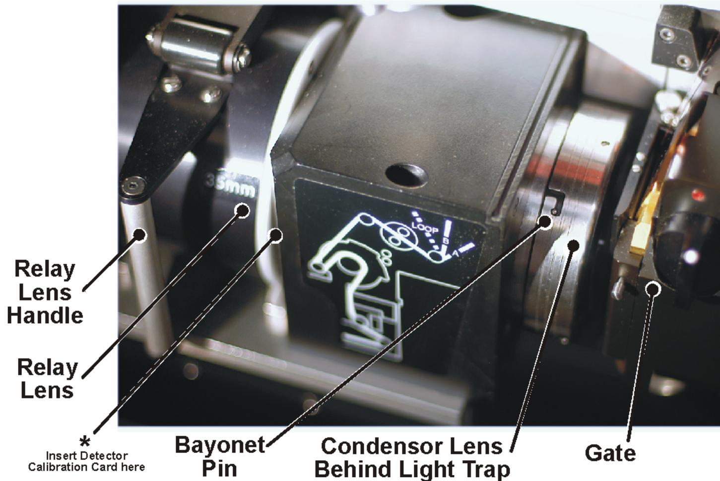
Figure 6 Oliver Condenser Lens
