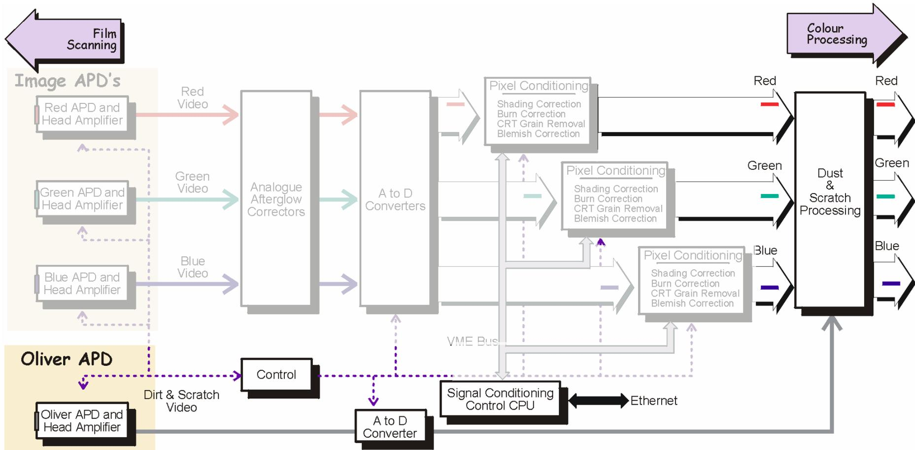
Figure 3 – Oliver Signal Path
